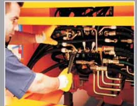
Separated hose system ensures economical, quick service and short repair period.
