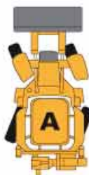
A-WAIST BREAK walk that increases maneuvering capacity during loading in narrow spaces
