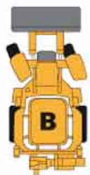
B-Steering from the FRONT WHEEL , used in road walk
