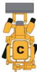
C-CRAB walk, used in excavations near walls and channels
