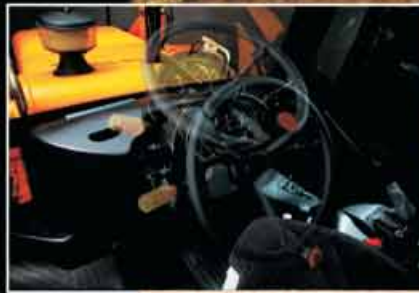
Steering wheel adjustable in all directions.
